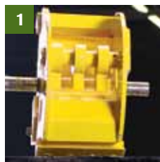
1- PATENTED MIXED ROTOR with 6 hammers with replaceable heads and 2 cutting blades
